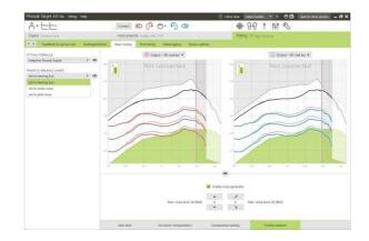
Within the drop down menu [Tinnitus balance shape] the default [Set to hearing loss] can be changed to [Set to white noise] or [Set to pink noise].
