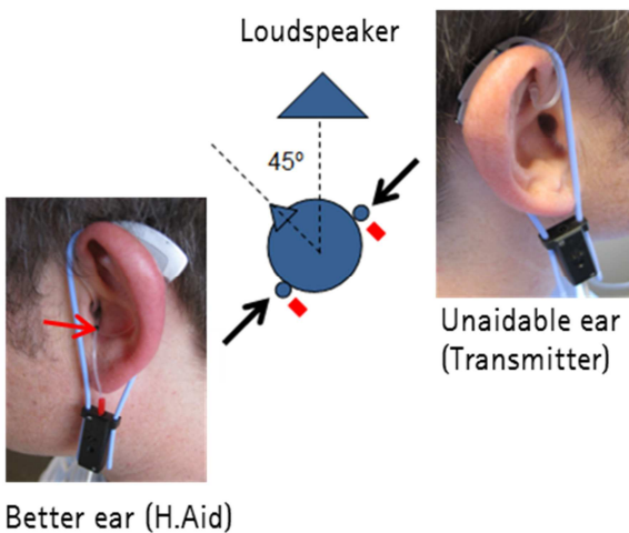
Fig. 7a: Equipment set-up for measuring the unaidable ear response.
