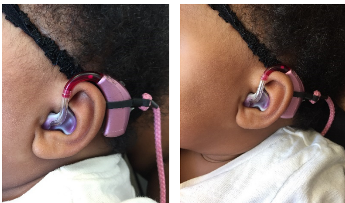
Figures 4. A loose fitting hearing aid with a standard earhook (left). An improved hearing aid fitting in which a mini earhook is used to improve positioning, retention and comfort over the ear (right).
