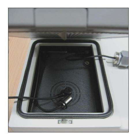
Box should be closed, but without changing the position of the microphone. Please hold the EasyBoom when closing the chamber.
