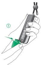
Attach the adapter to ZoomLink, then plug the MicroBoom cable into the microphone socket of the adapter.
