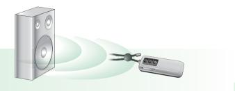
If the audio equipment does not have a headphone output socket, place ZoomLink in front of the loudspeaker of the television or the radio receiver. Then switch on ZoomLink and the television.
