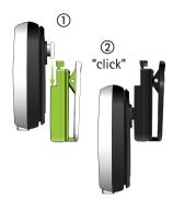
Fix the clip to the belt or trousers. Make sure the clip is secure.
