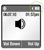
If the charging unit is removed from the inspiro, the segments in the battery symbol show the actual capacity.
