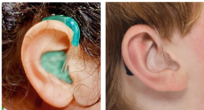
Figure 8. Traditional earhook and tubing on the left. SlimTube pictured on the right.
