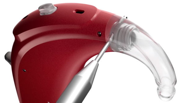
Figure 6. The Phonak tamperproof earhook being unlocked with the tool
