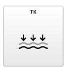
The amplification of very soft (G20) input sounds can be adjusted with the **[TK]** tuning tool. An increase of gain for very soft input sounds lowers the threshold knee point (TK) and vice versa.
