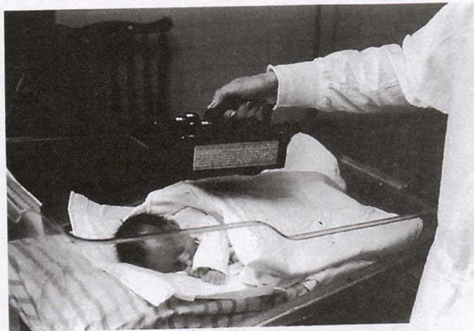
FIGURE 1-1. A specially designed battery-powered infant hearing screener used in the early 1960s known as the Apitron (from the auro-palpebral reflex, the involuntary body movement and eye blink resulting from sudden sound onset). The examiner presented a sudden onset narrow-band noise stimulus of 90 dB SPL followed by observation for the presence or absence of reflexive infant responses.
