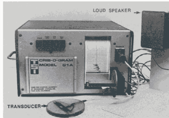
Figure 1. The Crib-O-Gram, which includes a central control unit with strip chart, a transducer, and a loudspeaker.
